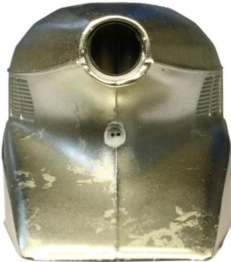
At the back of the body shell there is a moulded indent where the rear light should be. I drilled a 2mm hole just deep enough to fit the 0603 red LED. A 3mm drill was used to create a very small chamfer to allow gluing a homemade lens over the LED.
