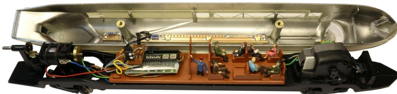
The bulb PCB was removed and the LED lighting PCB is hot melt glued into place as shown.
