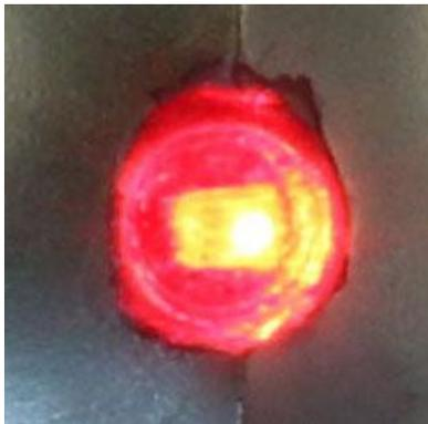
Close up with the red LED on. The homemade lens can be seen seated in the chamfered hole which reflects the red light.
