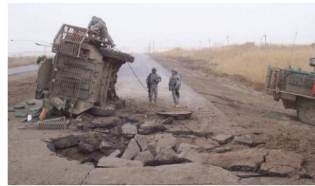
Figure 2: IED aftermath: a Stryker vehicle overturned by a buried IED blast (photo from www.army.mil)
